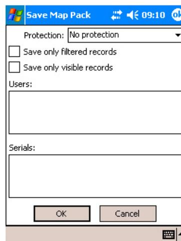
To limit the editing and printing layers select the „saving type” on the „Saving DMP” panel. The default setting is „No save”. Saving the DMP, it provides facilities to save the objects filtered through their attributes, or to save the geometry on the screen. The publication of the DigiTerra Map Package can be related to users, or serial numbers. (The user name and the serial number display the registration data).
